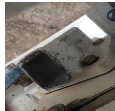
Broken arm with shallow weld.
